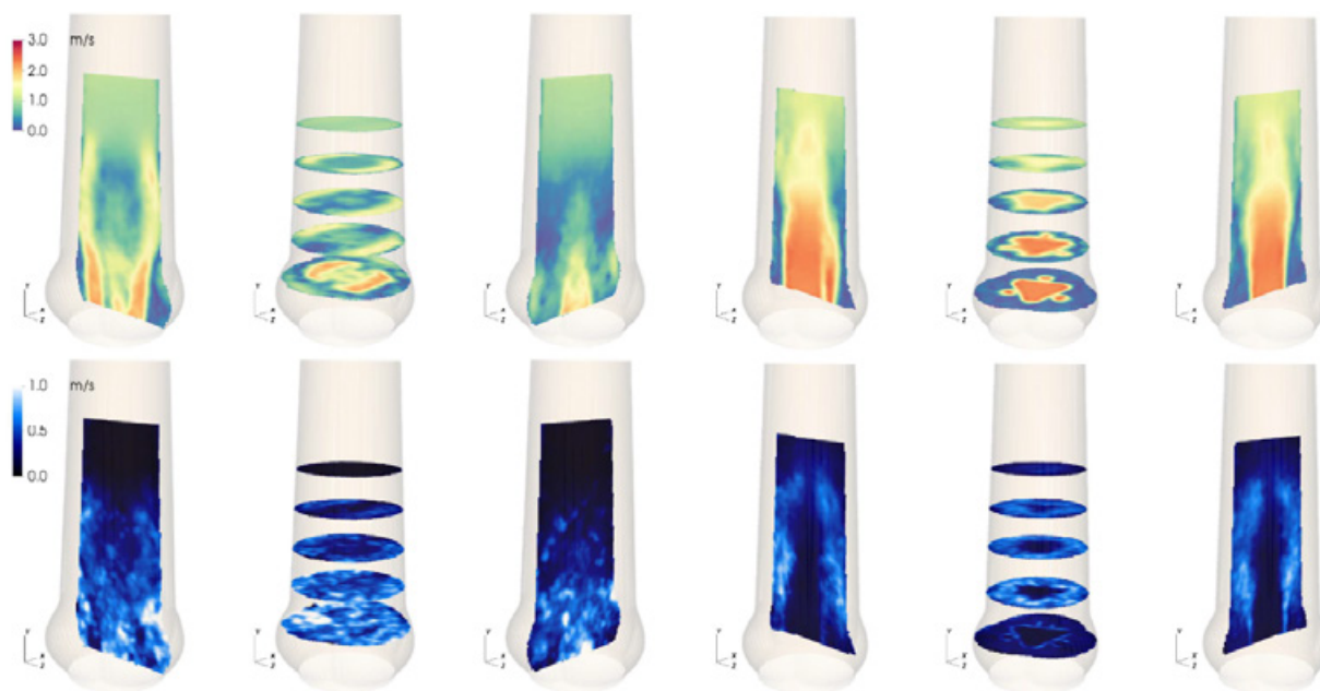
Mean velocity magnitude field \| \langle \mathbf{U} \rangle \| (upper panels) and RMS velocity fluctuation field U_{\text{rms}} (lower panels) at peak flow t = 0.15 s in BL (left panels) and TF (right panels) mechanical valve
